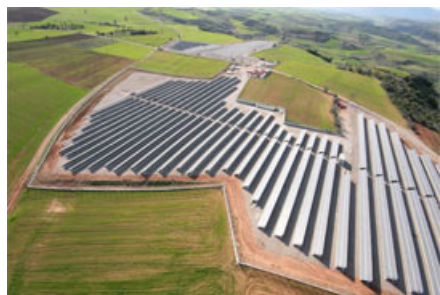
Greenfield PV plant in Thiva (approx. 50 km north of Athens) with 12.400 solar panels and a capacity of 2 MW, one of the biggest Greek solar power plants.
