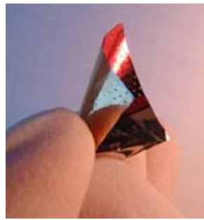
Left: Photo of a 30 cm x 30 cm module of dye-sensitised solar cells held against the sun. The module was sealed by a thermal process developed at the Fraunhofer ISE, during which so-called glass soldering (Glaslote) is affixed with screen-printing (glass with particularly low heat distortion temperature). Right: Organic ISE solar cell on flexible substrate (not encapsulated). Source: Fraunhofer ISE
