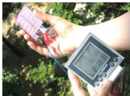
Flexible, organic solar cells manufactured at the Fraunhofer ISE. Organic solar cells of the University of California in Santa Barbara (UCSB). Sources: ISE; UCSB
