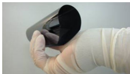
Left: Silicon Genesis produces 50 micron ( \mu\text{m} ) solar-cell substrates. Right: Konarka develops and commercializes "Power Plastic" a PV material that converts light to energy. Sources: Silicon Genesis; Konarka
