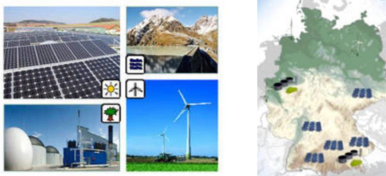
The Combined Power Plant consists of three wind parks (12,6 MW), 20 solar power plants (5,5 MW), 4 biogas systems (4,0 MW) and the pump storage Goldisthal (Output: 1.060 MW; Storage: 80 hours, i.e. 8480 MWh). Photos: [www.kombikraftwerk.de](http://www.kombikraftwerk.de)
